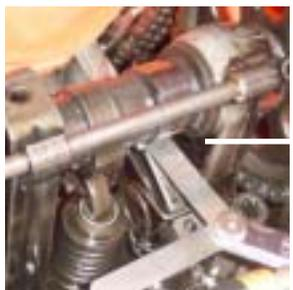
use feeler guages to measure the clearance between the camshaft and the rocker arm
