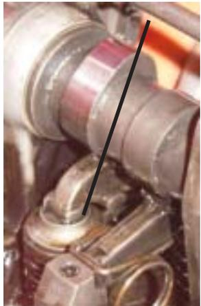
rotate the cam shaft\* so that the lobe opposes the valve
